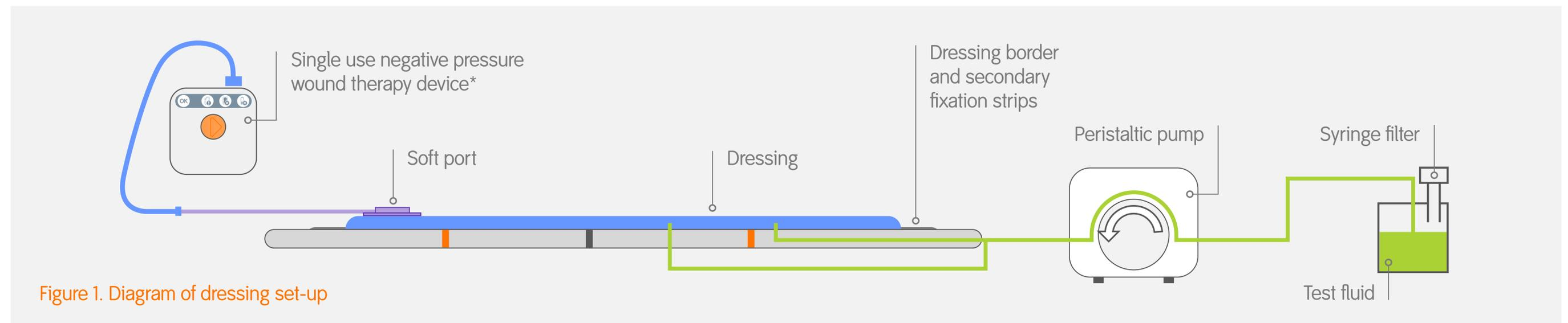
Figure 1. Diagram of dressing set-up
